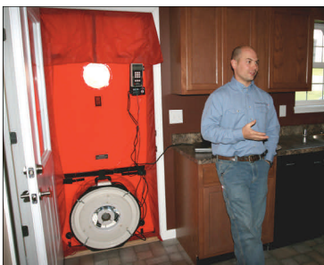
A blow door test verifies a home's energy efficiency.
