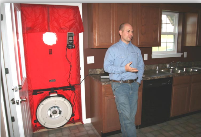
Blow door test demonstrates energy efficiency of the home. (photo by Ann Olson)
